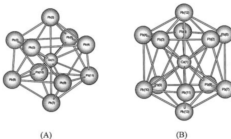
**Figure 4.** Possible structures of the  $[\text{CoPb}_{10}]^-$  and  $[\text{CoPb}_{12}]^-$  cluster anions. (A) bi-capped tetragonal antiprism structure of  $[\text{CoPb}_{10}]^-$ ; (B) icosahedral structure of  $[\text{CoPb}_{12}]^-$ .
