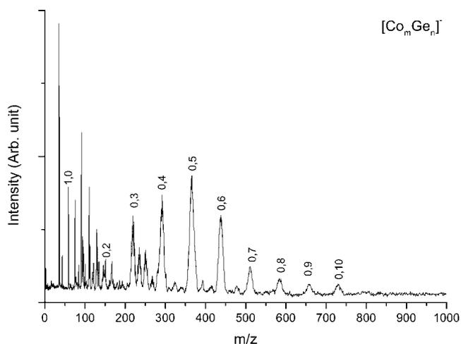
**Figure 3.** TOF mass spectrum produced by laser double ablation on samples Co and Ge.
