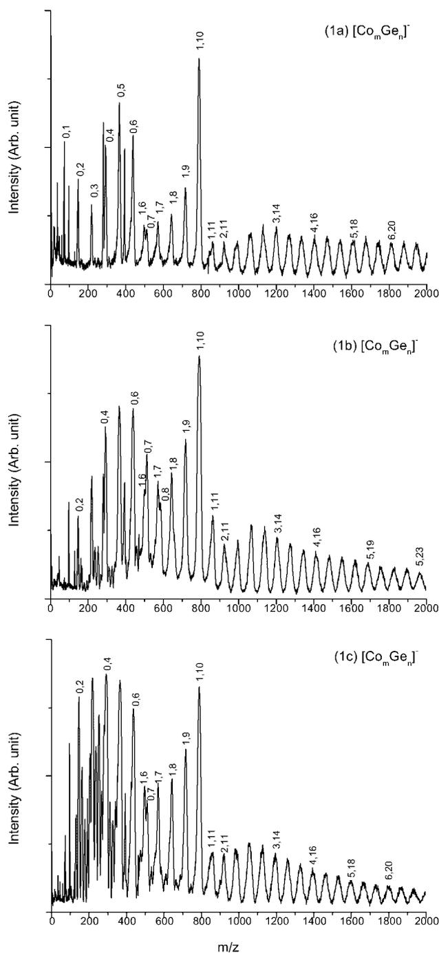
**Figure 1.** TOF mass spectra of Co/Ge cluster anions  $[\text{Co}_n\text{Ge}_m]^-$  produced by laser ablation on mixed samples of Co and Ge with different atomic ratios and laser powers. (a) Ge/Co = 1:1, laser power  $9.77 \times 10^7 \text{ W/cm}^2$ ; (b) Ge/Co = 4:1, laser power  $8.76 \times 10^7 \text{ W/cm}^2$ ; and (c) Ge/Co = 1:4, laser power  $1.01 \times 10^8 \text{ W/cm}^2$ .
