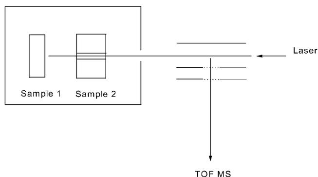
**Figure 2.** Laser double ablation reactor.
