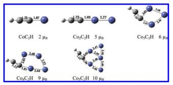
**Figure 4.** Optimized geometries of the most stable isomers of neutral  $\text{Co}_n\text{C}_2\text{H}$  (n = 1-5).
