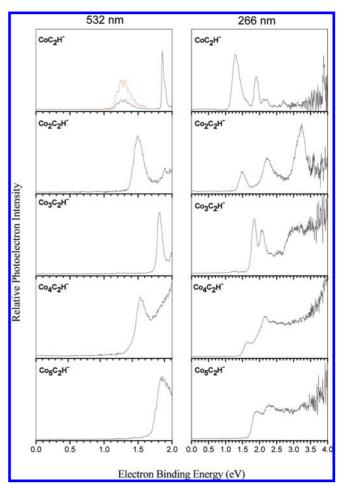
**Figure 2.** Photoelectron spectra of  $\text{Co}_n\text{C}_2\text{H}^-$  (n = 1-5) cluster anions recorded with 532 and 266 nm photons.
